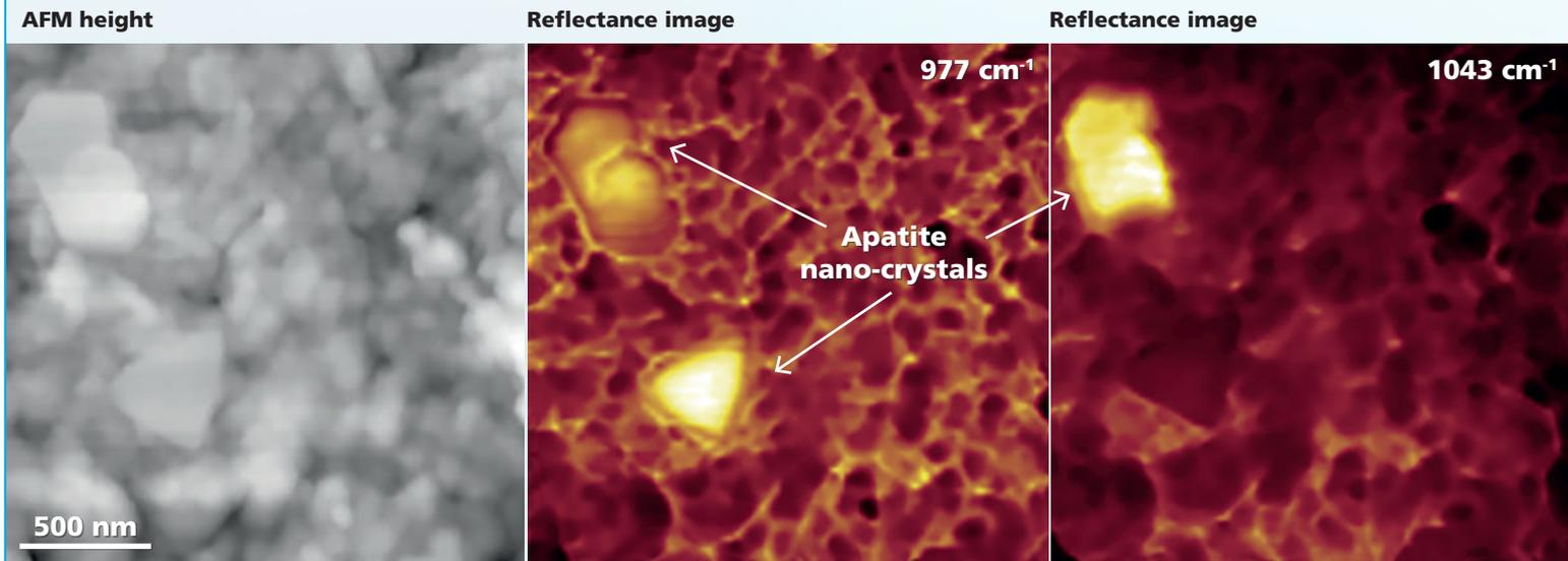
IR nanoscopy reveals nature's biochemical control of the mechanical properties of bone
