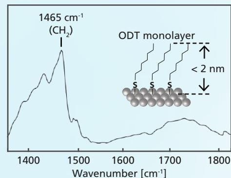
nano-FTIR demonstrates the effectiveness of ODT as corrosion inhibitor
