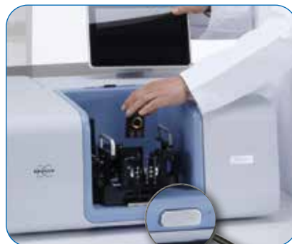
Sufficient space, even for bulky accessories in QuickLock™ mount with lock and release button in front.
